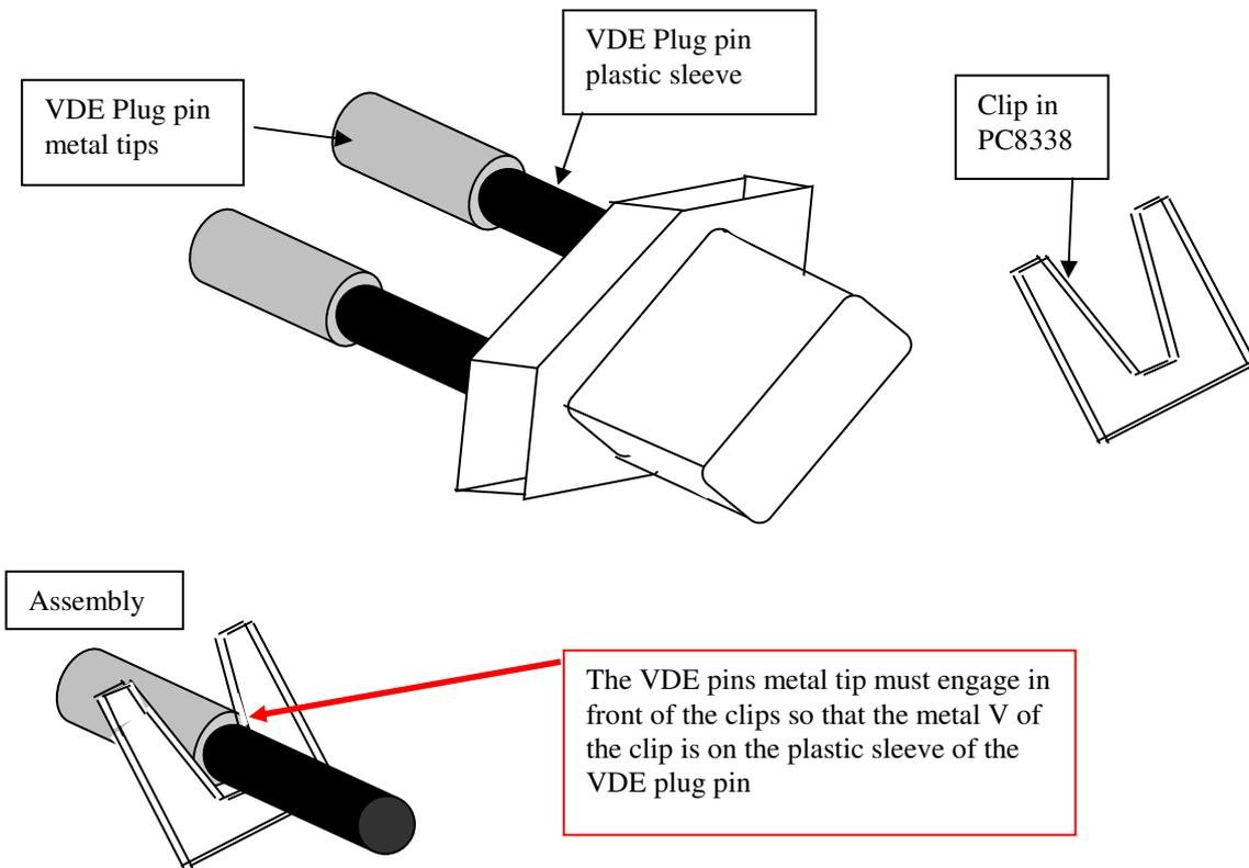
Once the VDE plug is correctly fitted close the cover and tighten the screw
