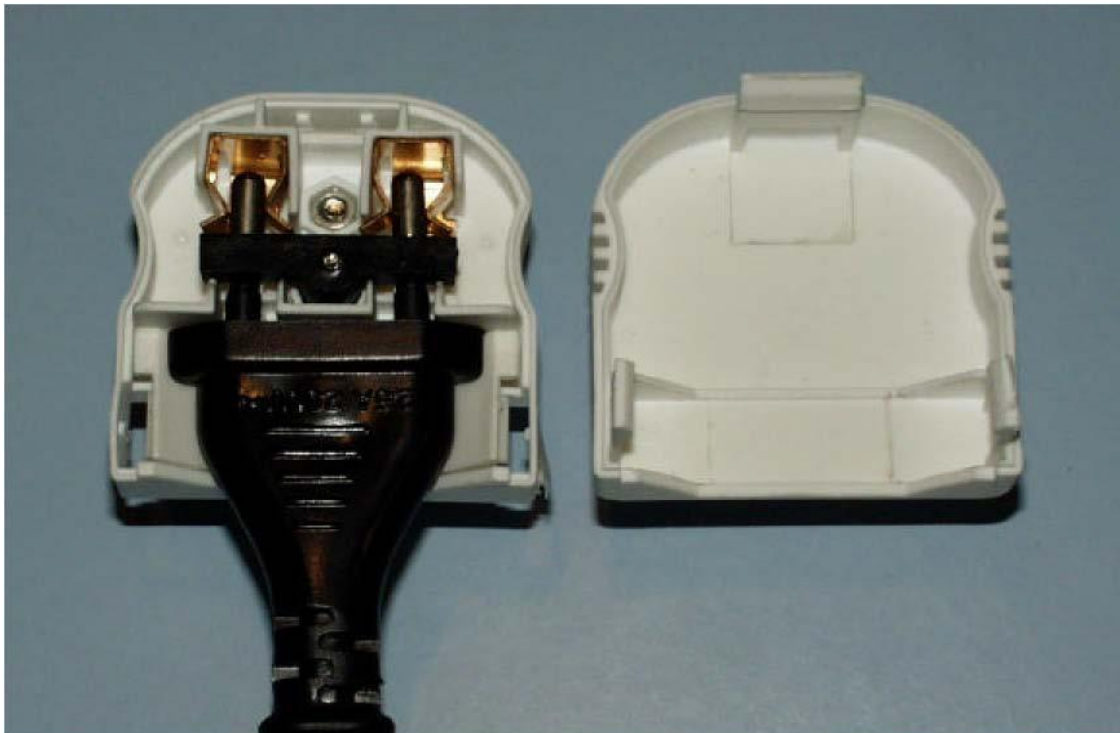
Internal view of CP3 showing CEE7 plug held in position
