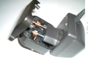
Torque screws to 0.4Nm (4.08Kgf.cm)
