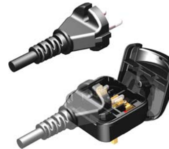
Diagram 2 Get plug and install in to clips, fit plug into SAP as shown and close lid, see diagram 3.
