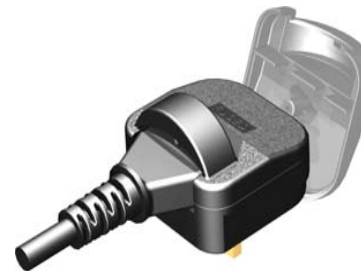
Diagram 3 Close lid SAP is now ready to screw up. Tighten screw in base to a torque of 0.5 Nm (Maximum)
